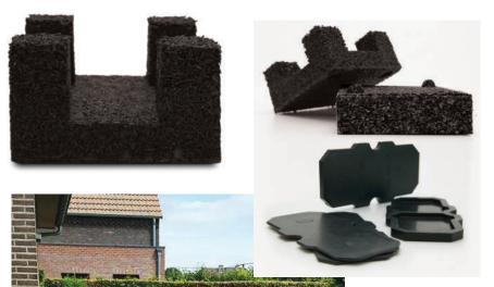
The outside area where the decking is to be installed does not have to be an even surface as the InstaCradle system is adjustable in height and can be levelled on site. Combinations of 2mm and 5mm cradle packers, with 10mm and 30mm interlocking base packers for more difficult areas, are used to alter the cradle height and ensure that the decking surface is completely level.
